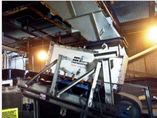
Custom-engineered transfer chutes confine the material stream and reduce air entrainment, helping to minimize spillage, abrasion, dust and premature wear.
