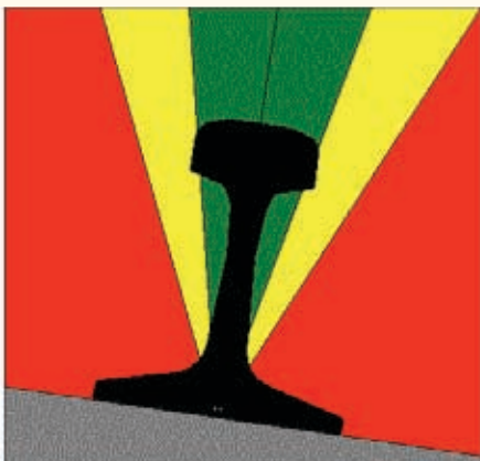
Figure 4. Rail cant exception thresholds.
