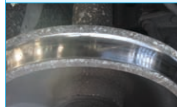
Wheels Conditioned by Sintered Shoe
