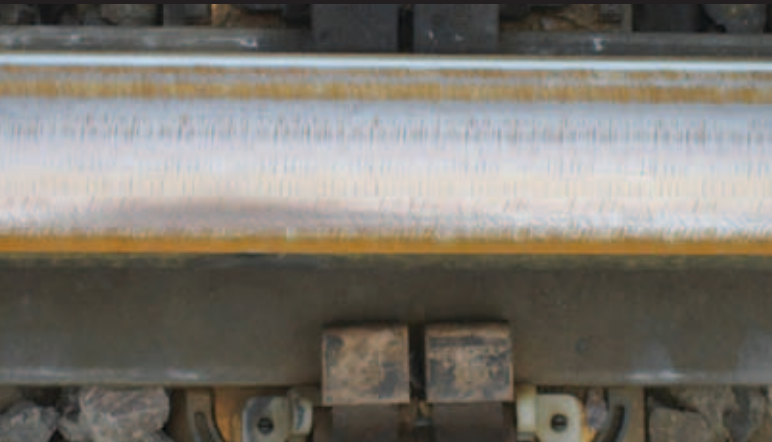
Figure 3b. UP keeps the rail free of spalls with 35- to 40-mgt cycles.
