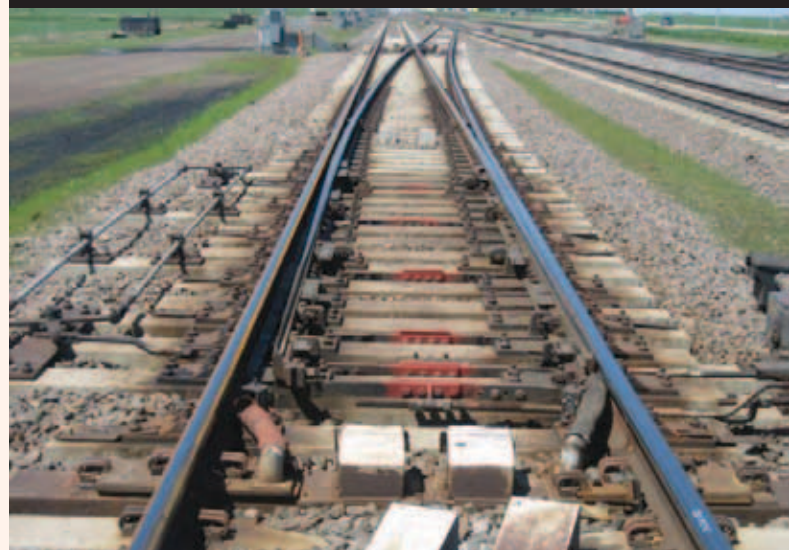
Figure 4. A crossover on the heavy-tonnage Kearney Sub, the dividing point at which loaded coal goes to either Kansas City or Chicago.
