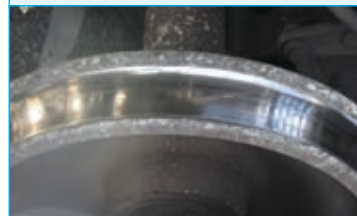
Wheels Conditioned by Sintered Shoe
