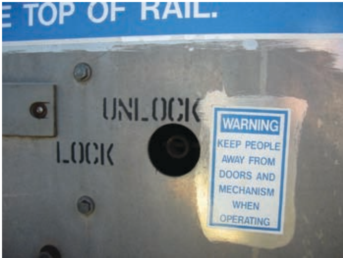
TYPICAL MANUALLY OPERATED MECHANISM THAT REQUIRES A TWISTING MOTION.
