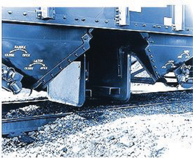
MODERN VERSION OF MANUALLY OPERATED DOOR SYSTEM.
