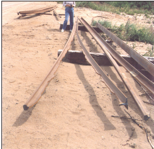
Figure 3. Rail containing high residual stress.
