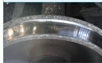
Wheels Conditioned by Sintered Shoe
